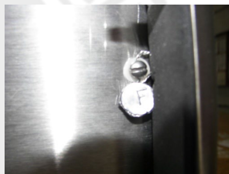
Sealing of Panel Mount
