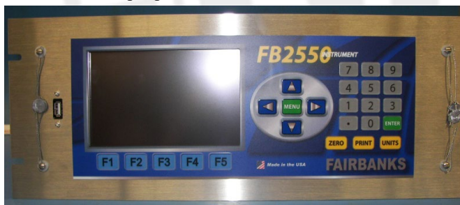
Rack Mount Option (Sealing of Front)
