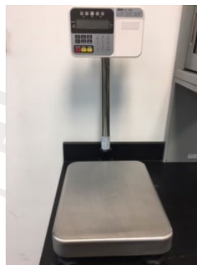
HV-60KC (60 kg) with pole mounted indicator
