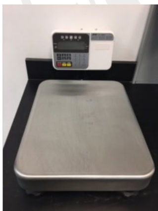
HV-60KC (60 kg) with remote cabled indicator
