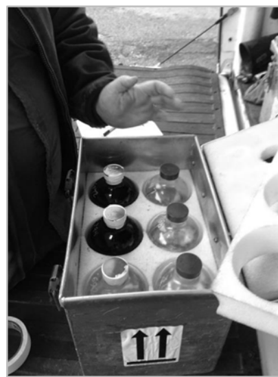
Figure 13b. Sample Box Showing Insulation.
