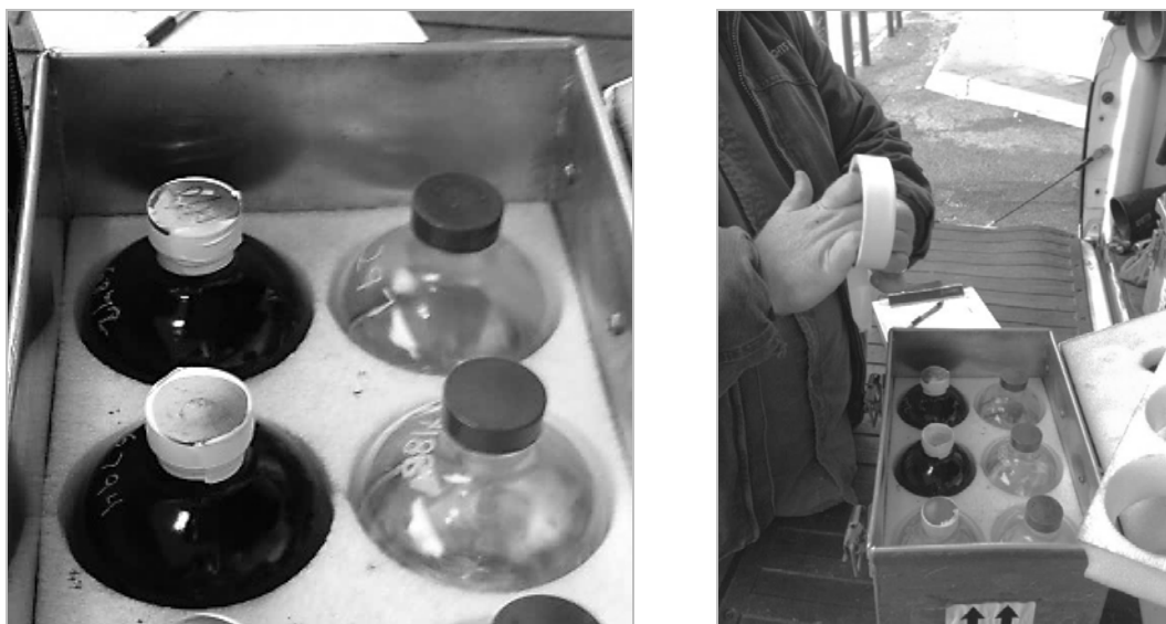
Figure 19. Sealing Tape Applied to Amber Sample Bottles
