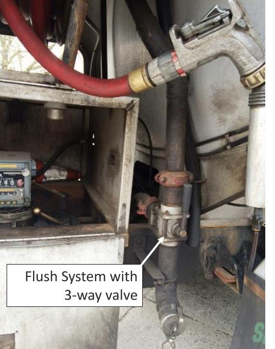
Fuel delivery truck owners have made their own manifold flush systems to improve safety for their drivers. While the intention was good in this example, the 3-way valve shown makes it unclear if the flush system is on or off. Situations like this raised the original need for regulations to prevent both intentional and unintentional fraud during flushing.
