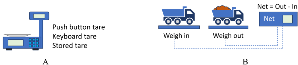
Figure 1: Tare operation (A) versus a calculated weight value (B)
