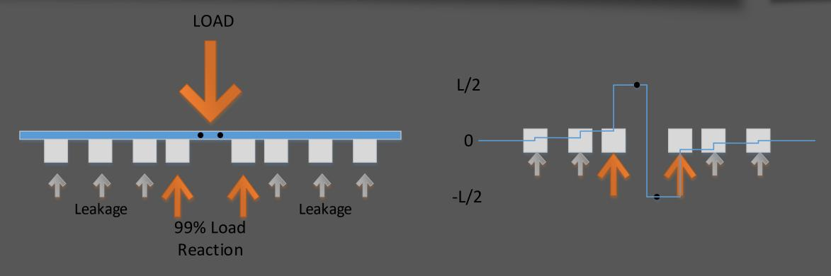
Sensor measures L/2 shear regardless of leakage.
