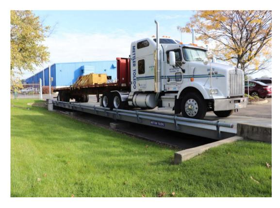
Capacity: 100'000 lb Increment (d): 20 lb CLC: 100'000 lb Accuracy Class: III L Speed Range: 1-5 mph Maximum Speed Change: 2 mph Max Wheelbase: 60' Vehicle Direction Capability: Uni-directional Dimensions: 70' x 11' Approach: 11' in plane, 70' straight
