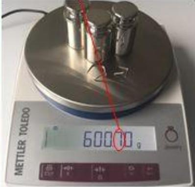
Scale with  $e = d$  & - Scale with  $e = 10d$  METTLER TOLEDO | 10
